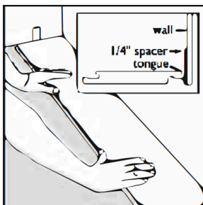
Begin the installation in the left hand corner against the wall. Place the plank a minimum of 1/4" from the left wall. Use the installation spacers throughout all perimeter area to insure the correct expansion space is maintained.
